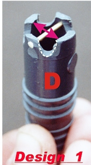
After cutting grooves and inserting bar. Dimension A is also shortened. After Insertion of brazing rod grind flat with angle grinder or sander.
